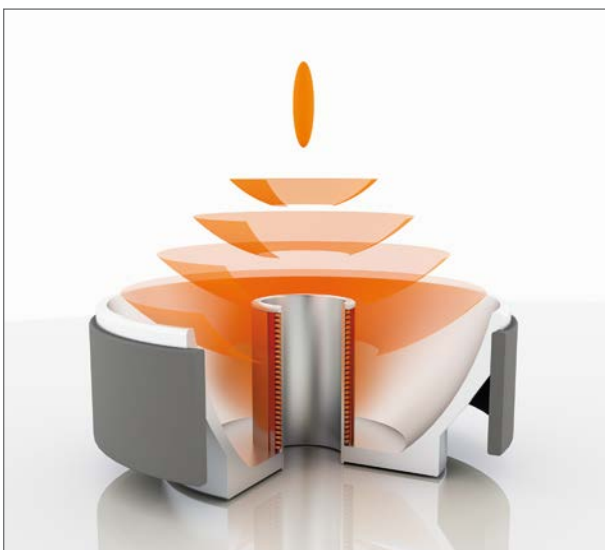
Fig. 4: Shock wave generation
