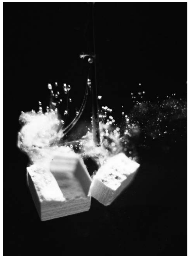
Fig. 8: Effect of a focused shock wave on an artificial stone
